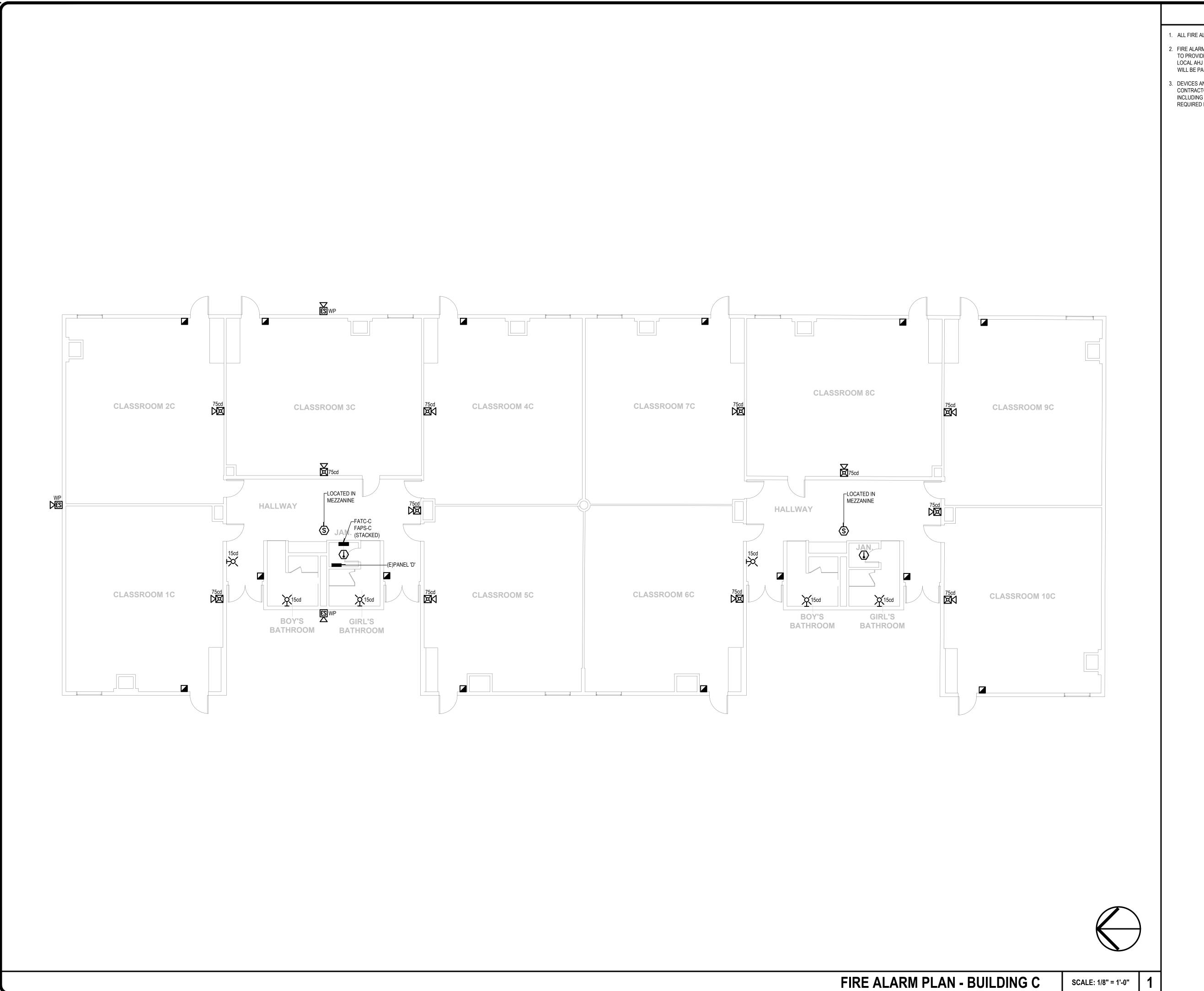
1. ALL FIRE ALARM WIRING SHALL BE INSTALLED IN CONDUIT SYSTEMS.
